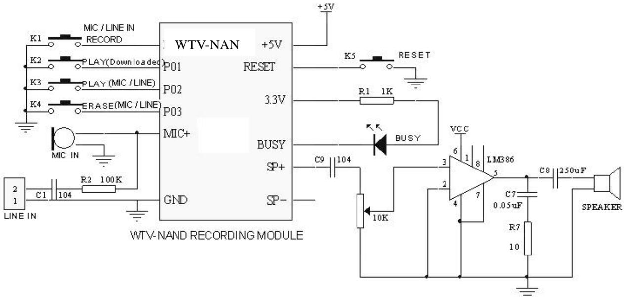
Circuit description : Key mode , P00 ,P01 ,P02 ,p03, corresponding key K1, K2, K3, K4 default as MIC/LINE IN record , PLAY (downloaded voice ) , PLAY (MIC/LINE IN recorded voice ) , ERASE (MIC/LINE IN recorded voice ) individually . BUSY output also for playing busy , low level at play or record status. Microphone connect to “MIC+”, LINE IN connect to “MIC+” after go through C1 and R2 . Reset connect to K5 , negative edge trigger and low level (50ms) can trigger to reset .
