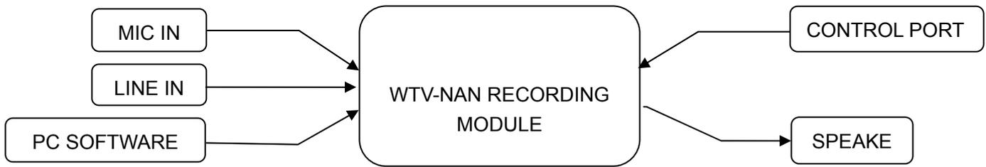
Description: Record voice to WTV-NAN module by MIC, LINE or PC software. Trigger module to play voice by control port. Support Samsung and Hynix 16MByte to 256MByte NAND-Flash .
