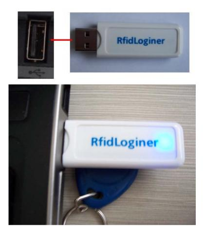
When plug the YHY202D reader to the PC's USB port, the system will recognize it as HID keyboard device.
